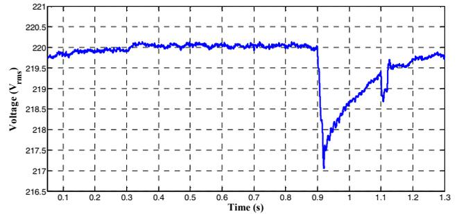
Fig. 11. Voltage profile under sudden load changes.
