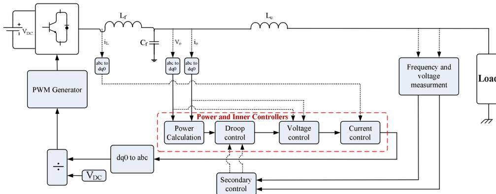
Fig. 3. Control structure of the IIDGs
