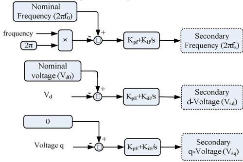
Fig. 6. Secondary voltage magnitude and frequency controllers
