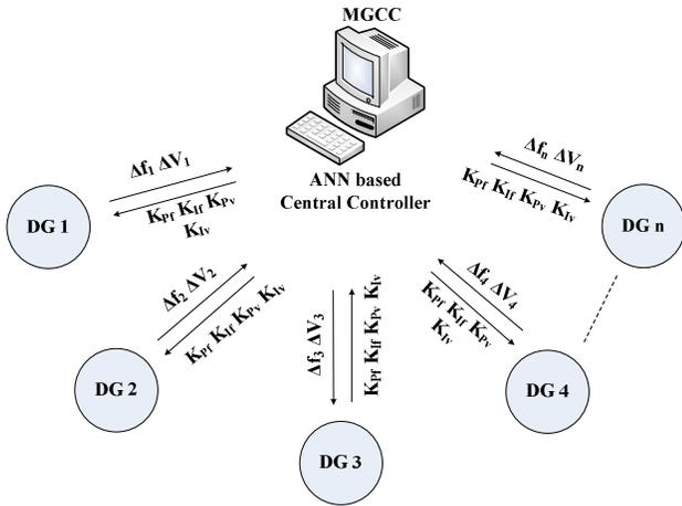
Fig. 11. Overall structure of online central controller.
