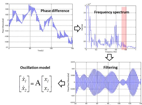
Fig. 3. Oscillation model estimation using phasor measurement
