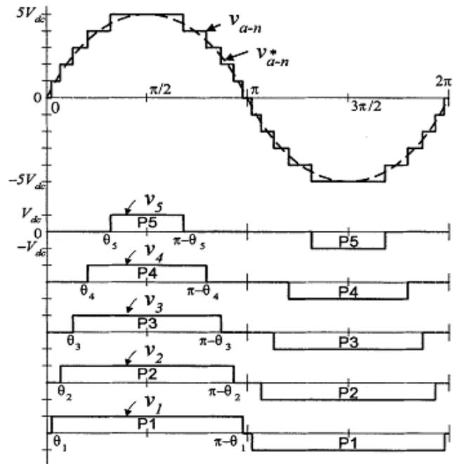
Fig. 1. CHB multilevel inverter and its output voltage [10]
