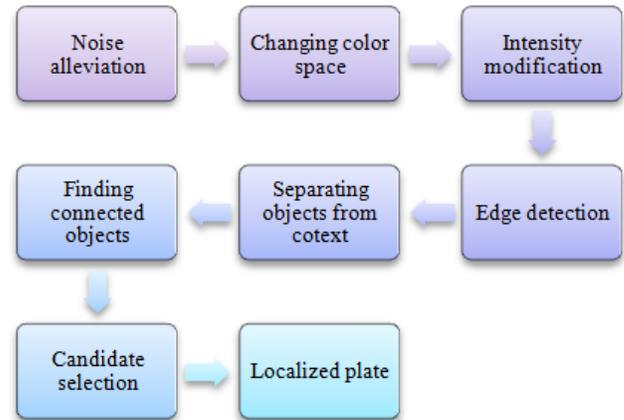
**Figure 1. Image plate localization process**
