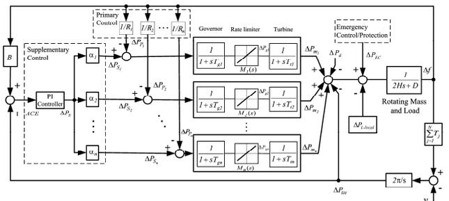
**Fig. 1.** Modified frequency response model for emergency conditions
