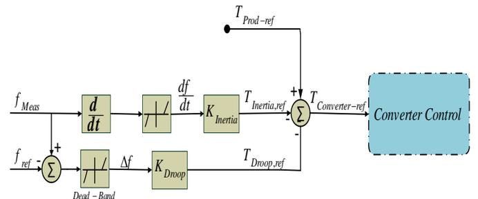
Fig. 2. Proposed control strategy for DFIG wind turbines.
