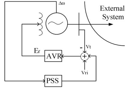
Fig. 2. Generator with conventional AVR and PSS
