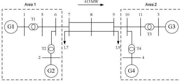
Fig. 1. Test case power system
