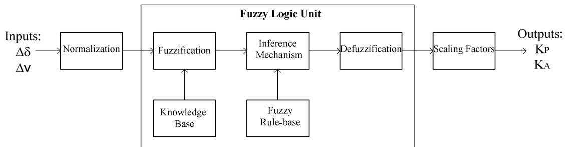
Fig. 3. A step-by-step scheme for fuzzy controller
