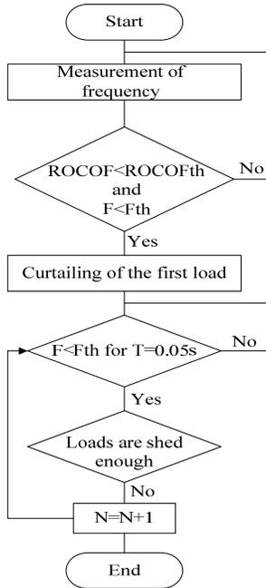
Fig. 10: Flowchart of the proposed load shedding algorithm
