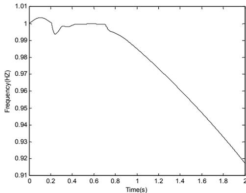
Fig. 11: Frequency of MG before load shedding
