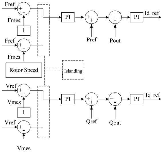
Fig. 3: Active and Reactive Controller
