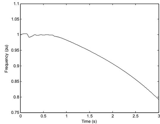
Fig. 10: Ferequency of MG before load shedding
