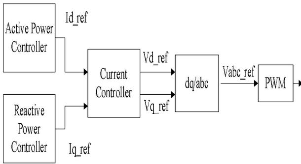
Fig. 5: Control Structure
