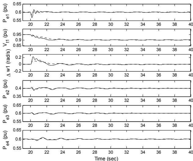
Fig. 6: System response for a 0.05 pu step change at the voltage reference input of unit 1; Solid ( $H_\infty$ -SOF), dotted ( $H_\infty$ -Dynamic).
