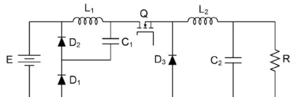
Fig. 1. QBC with a single switch.
