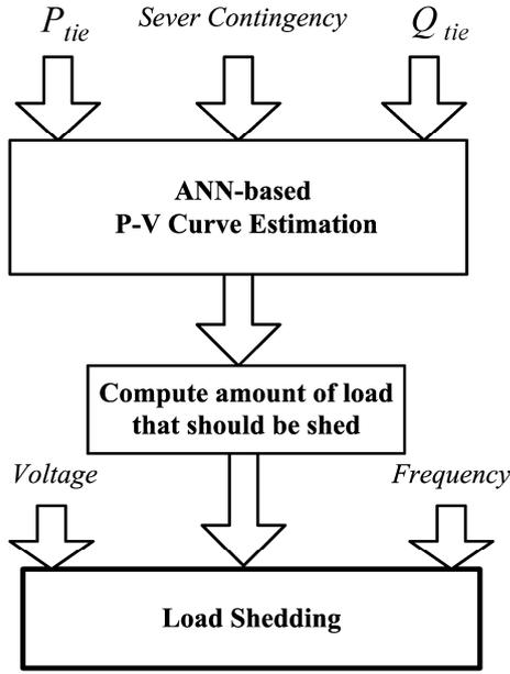
Fig. 5 The proposed intelligent based emergency control scheme.
