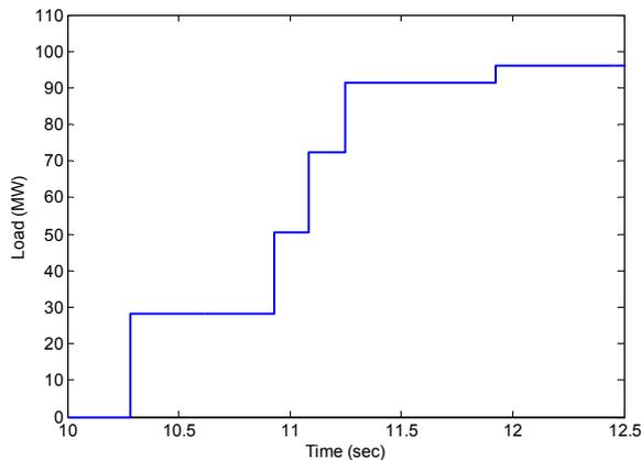
Fig. 8 The LS steps and amount of load that should be shed in each step in the case of G2 outage.
