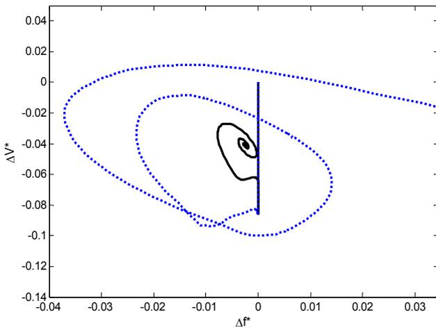
Fig. 6 Phase trajectory for post-contingency stability analysis; stable (solid) and unstable (dotted) post-contingencies.
