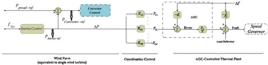
FIGURE 4 Proposed control scheme for wind-conventional power plant
