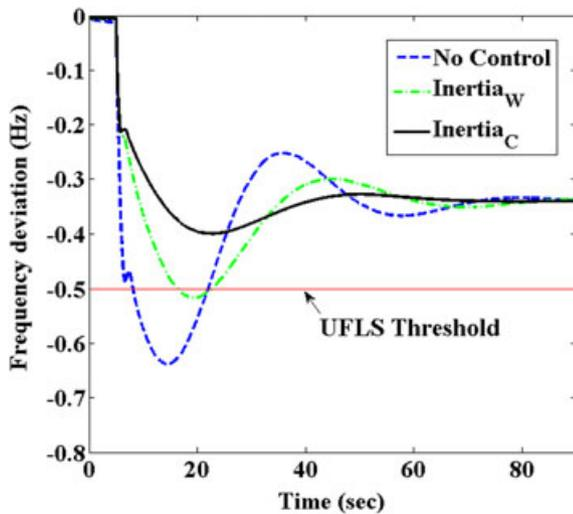
FIGURE 9 Frequency response for Scenario 3 (40% wind power penetration)
