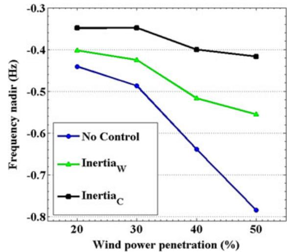
FIGURE 11 Impact of wind power contribution on the frequency nadir
