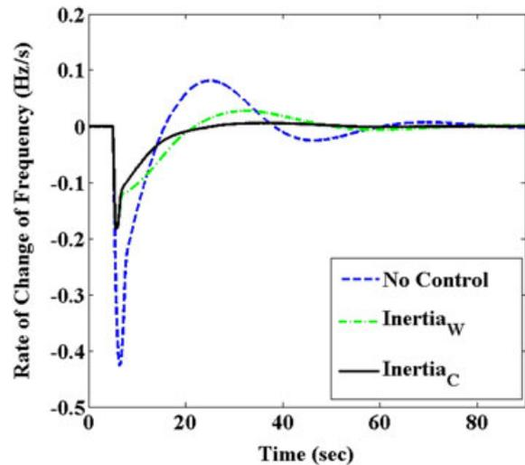
FIGURE 16 Rate of change of frequency response for Scenario 4 (50% wind penetration)
