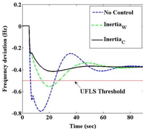
FIGURE 10 Frequency response for Scenario 4 (50% wind power penetration)
