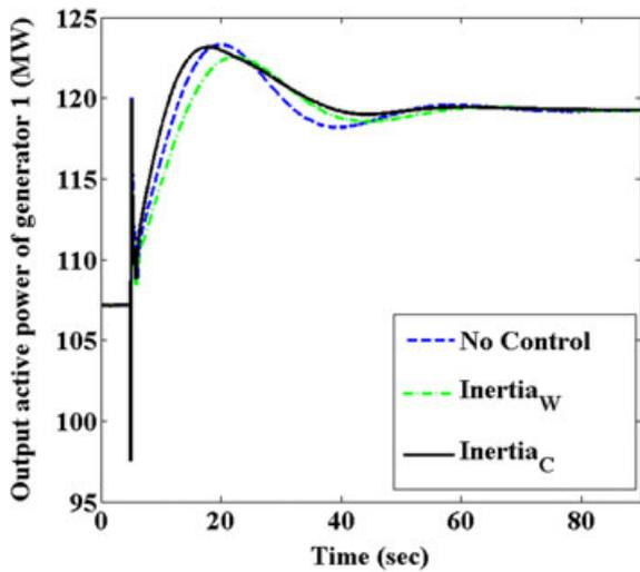
FIGURE 13 Output active power response of generator 1 for Scenario 1 (20% wind penetration)
