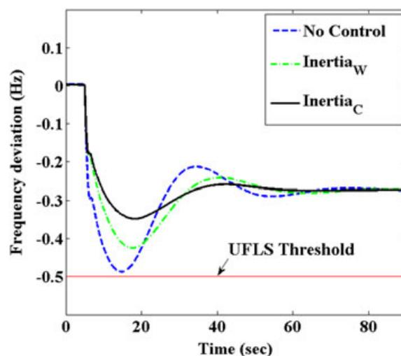
FIGURE 8 Frequency response for Scenario 2 (30% wind power penetration)
