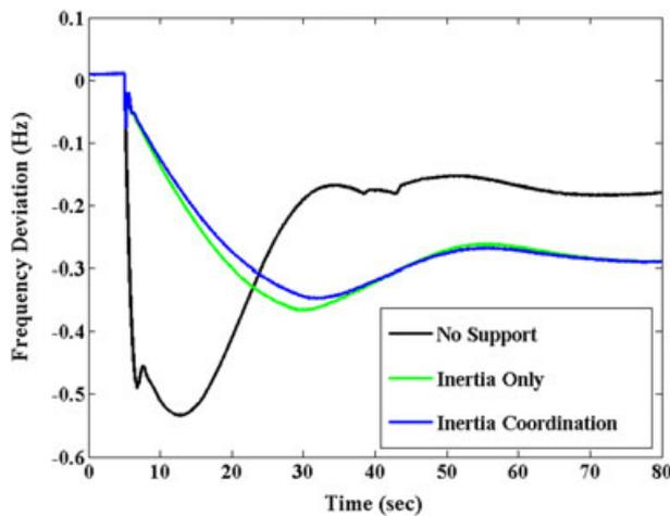
FIGURE 18 Frequency response for 50% wind power penetration
