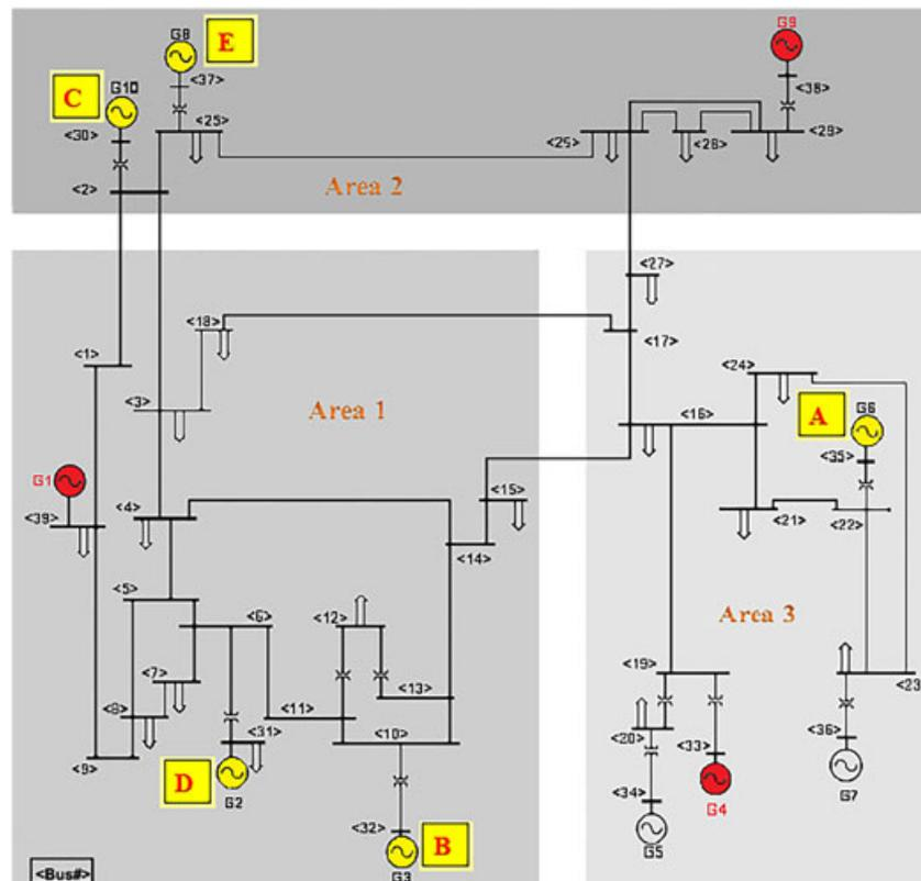
FIGURE 5 Single diagram of New England test system
