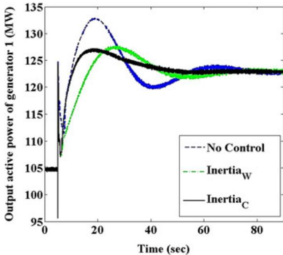
FIGURE 14 Output active power response of generator 1 for Scenario 4 (50% wind penetration)
