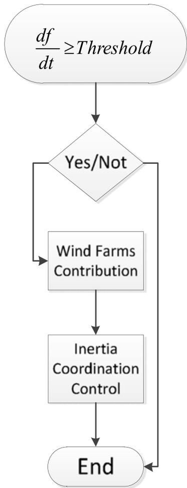
FIGURE 6 Flowchart of the control procedure
