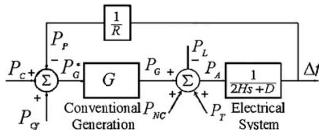
FIGURE 3 Power system model with presence of nonconventional generators<sup>19</sup>
