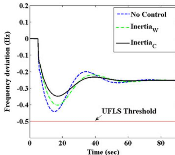
FIGURE 7 Frequency response for Scenario 1 (20% wind power penetration)
