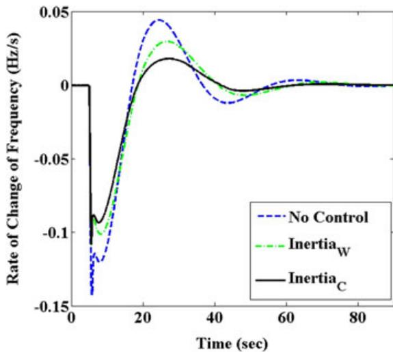
FIGURE 15 Rate of change of frequency response for Scenario (20% wind penetration)
