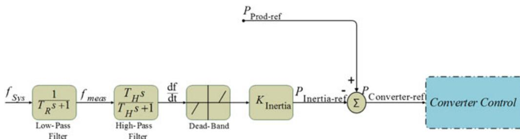
FIGURE 2 Structure of control strategy for DFIG-based wind turbine. DFIG, doubly fed induction generator
