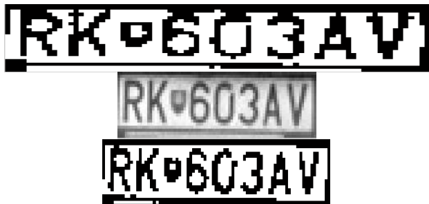
Figure 8. Local binarization against noises, up is binarized using global thresholding using Otsu method, bottom right is local binarized, bottom left is the input gray image
