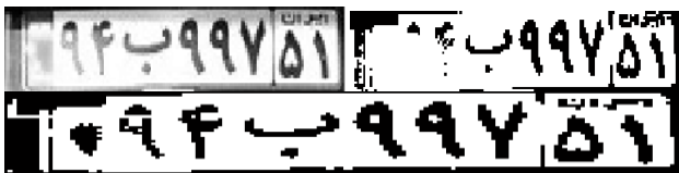
Figure 7. License plate binarization. Up left is the gray plate, up right binarized using Otsu method, bottom binarized using proposed method in section 4.2.3
