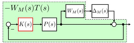
**Inverse-based Controller:**  $K_{\text{inv}}(s) = P^{-1}(s) \begin{bmatrix} \frac{900k}{s(s+30)} & 0 \\ 0 & \frac{900k}{s(s+30)} \end{bmatrix}$
