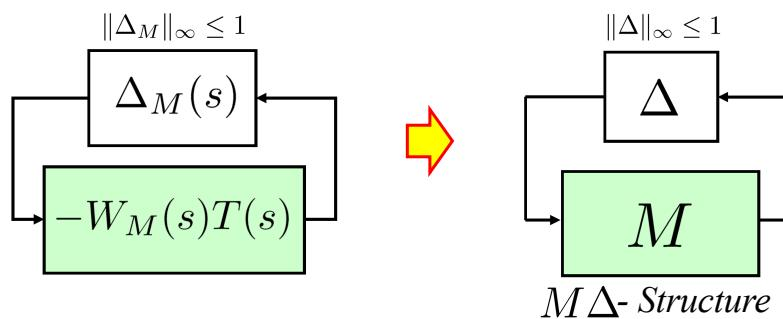
The closed-loop system is internally stable if  $M\Delta$  is stable and satisfies  $\|M\Delta\|_\infty < 1$
