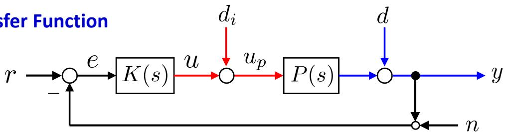
Loop Transfer Function at the input to the plant
