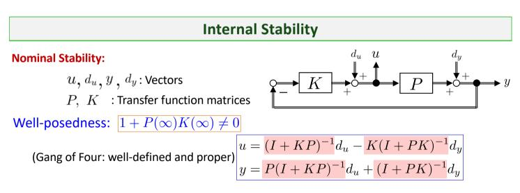
**Theorem:** Assume *P*, *K* contain no unstable hidden modes. Then, the feedback system in the figure is *internally stable* if and only if all four closed-loop transfer matrices are stable.
