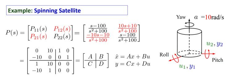
Inputs:  $u_1 u_2$  Torque Outputs:  $y_1 y_2$  Angular velocity
