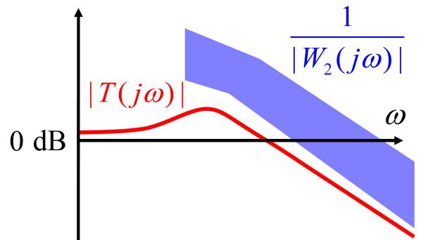
**Robust Stability:**  $|T| < \frac{1}{|W_2|}, \forall \omega \rightarrow$  Smaller T is better at higher W₂ frequencies
