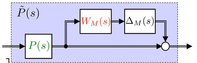
$$W_M(s) = w_M(s)I = \begin{bmatrix} w_M(s) & 0 & 0 \\ 0 & \ddots & 0 \\ 0 & 0 & w_M(s) \end{bmatrix}, \quad w_M(s) = \frac{\tau s + r_0}{\frac{\tau}{r_\infty}s + 1}$$
